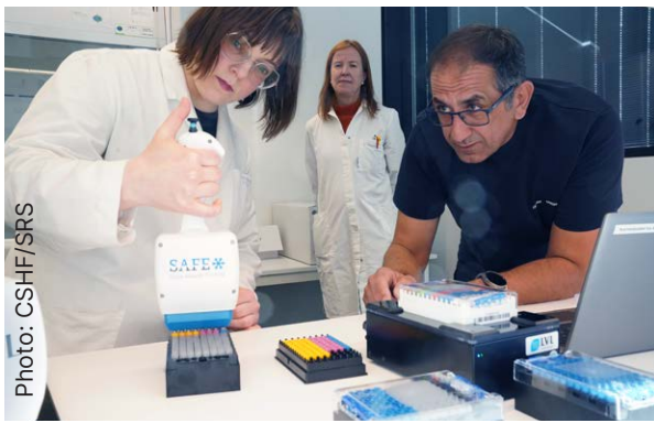
Product training at UiT. Showing the use of an LVL SAFE® Capper/Decapper to cap 8 tubes with color-customized caps, and an LVL rack reader that identifies each tube and position in the 96-tube rack by reading the 2D code at the bottom of the tubes.
