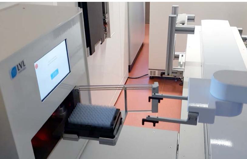
Automated LVL SAFE® 96-Channel Capper/Decapper in the automated process
